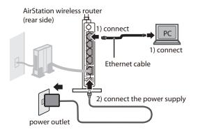
**5** Confirm the devices are connected correctly as the below diagram shows.
