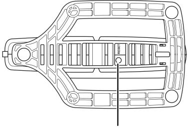
Hold down this button for 3 seconds. The AirStation will be initialized.
