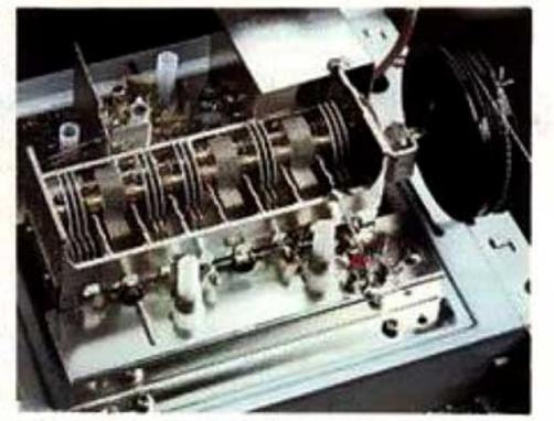
low NF (noise figure), combine to achieve optimum gain allocation and obtain a sensitivity to signals as faint as 1.5 µV (IHF).
