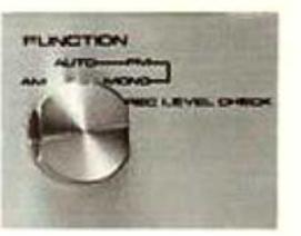
ment before you begin to tape an FM program (just set the recording levels to indicate -2dB on the deck's VUs). You may also wish to use the check level signal to determine proper speaker phase or to balance left and right channels.
